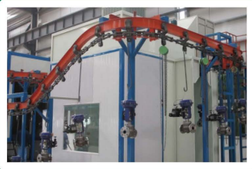
自动喷漆线 Automatic painting line
