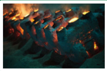
浇注、焙烤 pouring, baking
